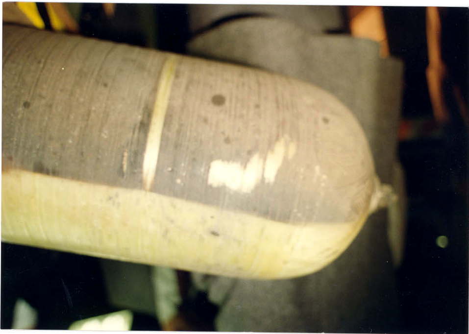
28. Brake Cable Rub Mark on the Rear of the Ruptured Cylinder
